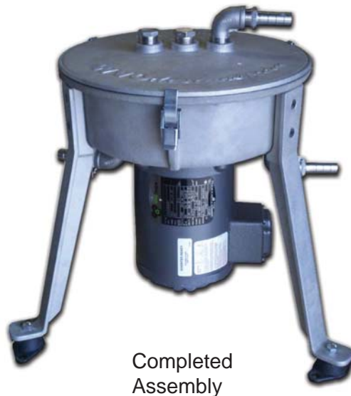
15. Apply High Temp Pipe Sealant to all male threads. Screw (1) Hose Barb into (1) 90° Elbow and (2) Plugs into Lid. Use (1) Hose Barb in place of (1) Plug if you are going to vent the Lid.
